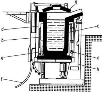
Figure 112. Layout of an induction crucible furnace [82]
