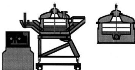
The temperature drop of the melt in the unheated Pouromat® system is limited to max. 1.5 K/min. This is enhanced by the shape of the pouring basin with a very small surface and the pneumatically actuated lid over the filling funnel.
