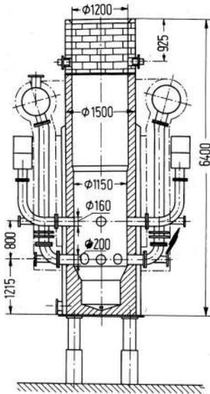
Figure 33. Furnace with secondary row of nozzles
