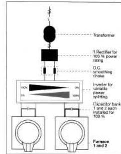
Figure 6: TWIN POWER circuit
