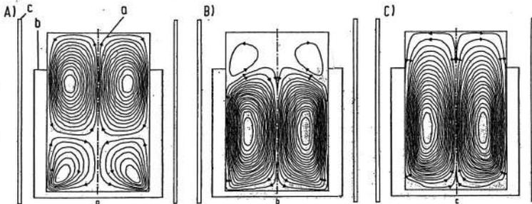
Figure 78. Flow field of a melt with single- and multiple-phase (travelling field) coil [73]
