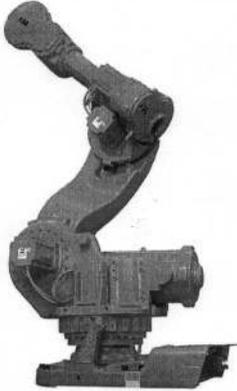
Figure 1: Angular-arm robot IRB 7600 with 500 kg load capacity.
