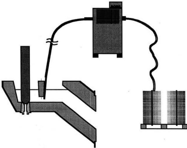
Fig. 9: Wire inoculation in the pouring spout
