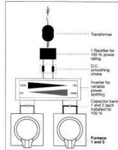
Figure 6: TWIN POWER circuit
