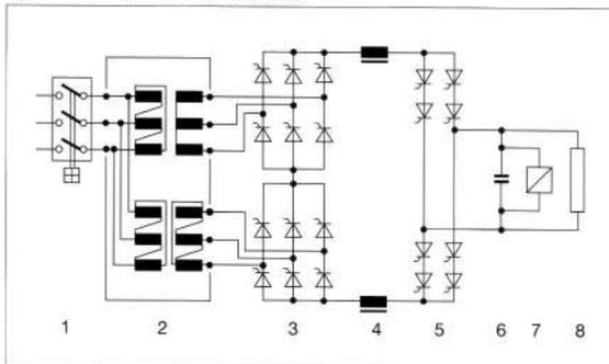
Figure 2: Block diagram of a thyristor converter (12-pulse)
