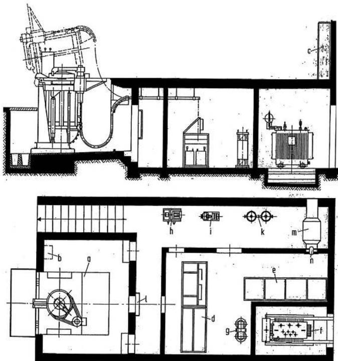
Figure 114. Layout of a complete system and installation plan for medium-frequency crucible furnaces [82].
