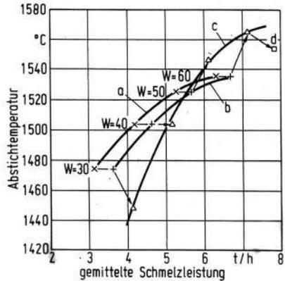
Figure 34. Iron temperature in relation to wind volume and added oil, coke percentage = 10%
