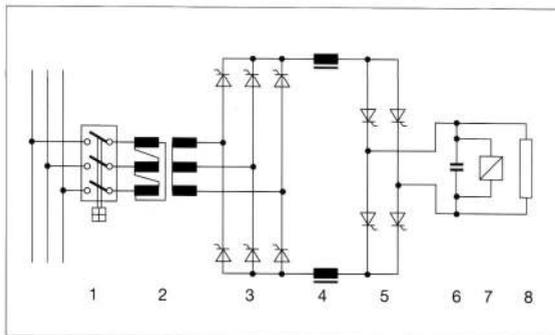
Figure 1: Block diagram of a thyristor (6-pulse)
