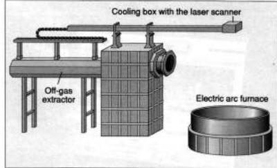
**Fig. 2.** Schematic diagram of the LaCam manipulator unit
