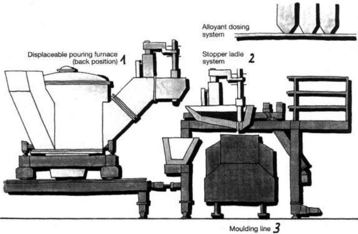
Fig. 15: Stopper ladle pouring system with pouring furnace and ladles arranged on a car
