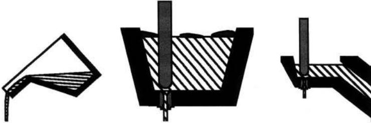
Fig. 3: Tilting ladle, stopper ladle, pressurized pouring system
