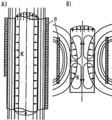
Figure 76. Principle of the induction crucible furnace [73]
