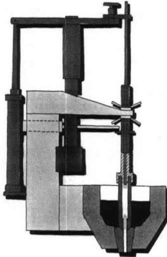
Fig. 10: ABB stopper mechanism with patented pouring nozzle cleaning device
