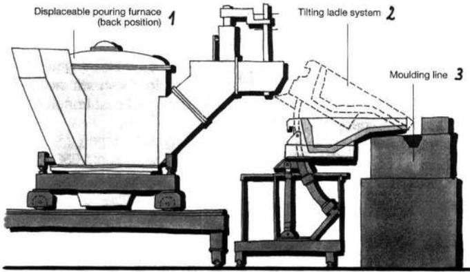
Fig. 13: Tilting ladle system with the PRESSPOUR® pouring furnace
