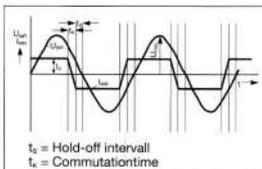
Figure 5: Time characteristic of the converter voltage  $U_{mn}$  and the converter current  $I_{mn}$
