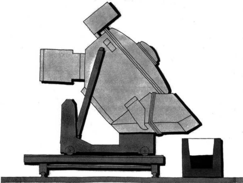
Fig. 2: Tilting of the PRESSPOUR<sup>®</sup>-furnace for total emptying
