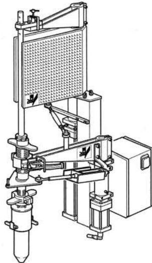
Fig. 6: Design of the ABB stopper system for automatic pouring.
