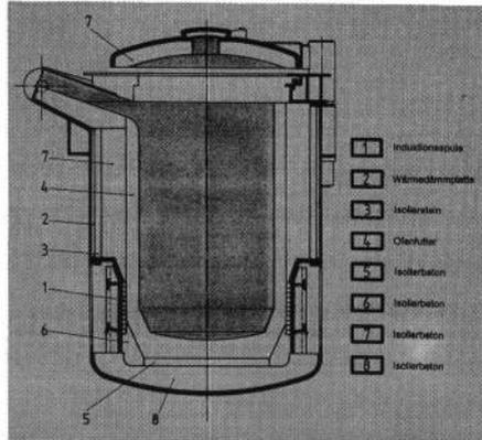
Figure 12: Crucible-type storage furnace with short coil
