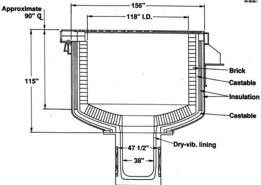
Fig. 1: Coreless inductor furnace
