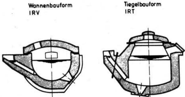
Figure 3: Cross-section through the vessel of a tub-shaped (left) and crucible-shaped channel-type furnace tub shape (IRV) - crucible shape (IRT)
